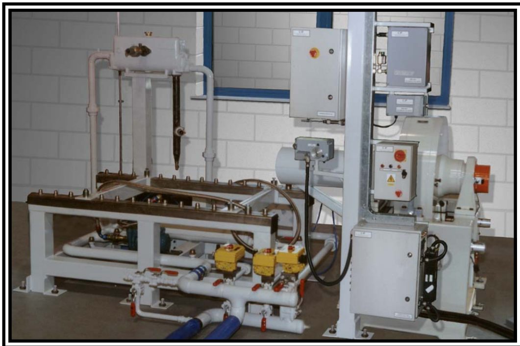
A typical VTB installation. This example shows an optional third temperature control module, API dynamometer with stool and FMS-400 fuel meter
